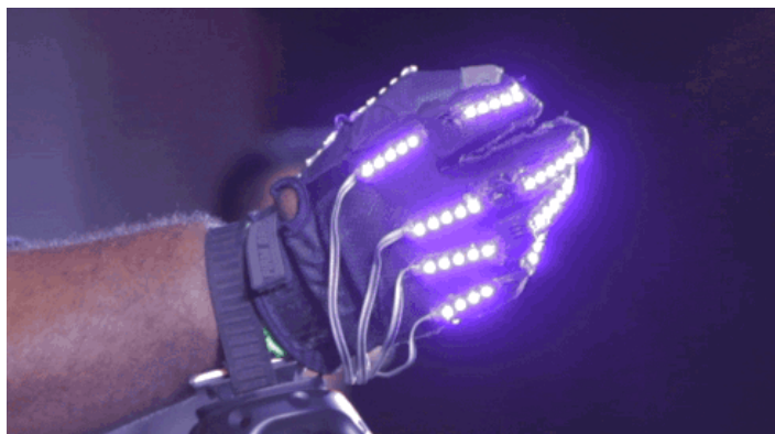
Above: Michael Ndubuisi '14 (left) and Ray Li '14 during a Vesium performance. Below, a detail of the suit's glove. Their music is created using this system, which makes sound through motion and gestures.
